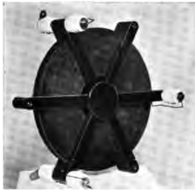
FIG. 28.—Protective inductance coil for transformer windings, etc. [See p. 82.]
